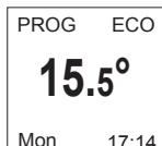
If the screen displays ECO PROG, you are in a programming range in ECO mode. By default, the ECO temperature is set to -3.5°C in relation to the COMFORT temperature.
