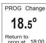
You may modify the ECO temperature; force the default setting between the Comfort temperature and the Eco temperature. "PROG Change" is displayed until the next Comfort window.
