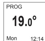
If the screen displays PROG, you are in a programming range in Comfort mode.
